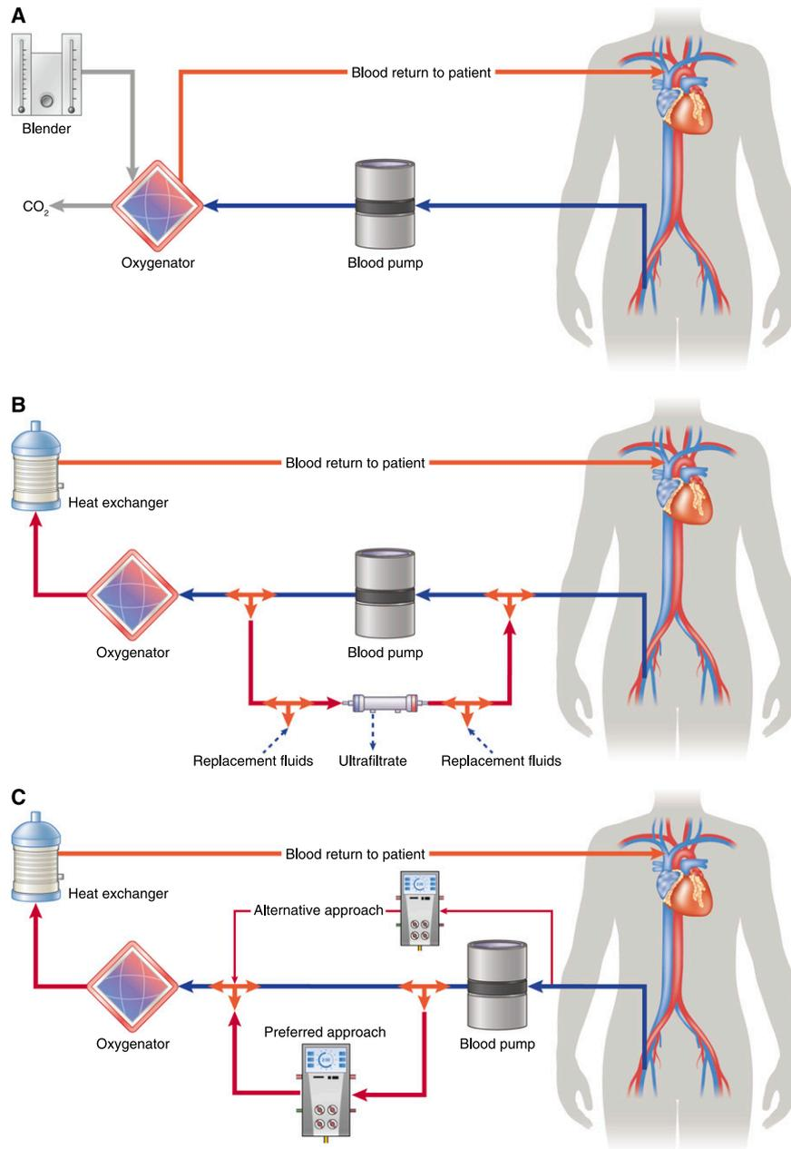
**Figure 1. | Schematic of an ECMO circuit.** Schematic of an ECMO circuit (A) incorporating either in-line hemofiltration (B) or a CRRT device integrated into the ECMO circuit, showing our preferred and alternative connections (C). CRRT, continuous RRT; ECMO, extracorporeal membrane oxygenation.
